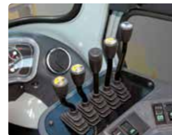
Quick Response of Operating Control Levers Only minimal operator's effort is required for precise, safe and productive control. (5-Lever, 6-Function : Standard) (5-Lever, 7-Function : Option)
