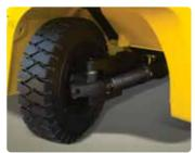
Fully hydrostatic power steering Key-locking fuel filler
